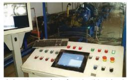
• hydrostatic testing of a pipe from 1.0 to 13.0 m in length with an outer diameter from 102 to 250 mm assembled with a coupling for sealing with a computer system for collecting and storing information; the maximum proof pressure is 75 MPa;
