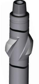
Stabilizers are intended to stabilize (improve) the operation of the guide section of the drill string by limiting the pipeline deflection, especially in the presence of caverns, dampening transverse (partially longitudinal and torsional) vibrations of the drilling tool at its contacts with the borehole wall.
