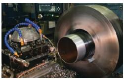
• thread cutting at the ends of pipes with an outer diameter from 102 to 245 mm;
