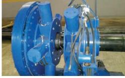
• coupling screwing-on with an outer diameter from 102 to 245 mm on a specialized machine with a thread tightening control;
